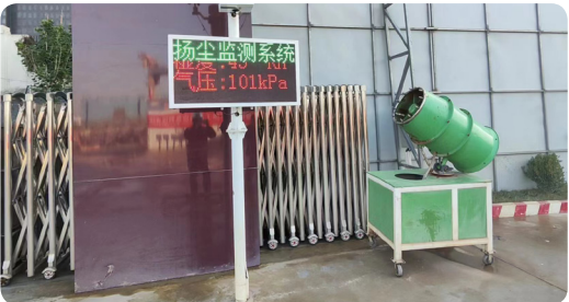
▲ Dust Monitoring Instrument & Dust Suppression Cannon
